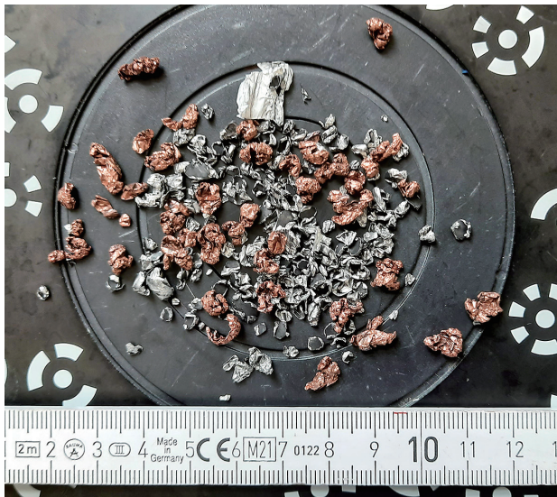
Fig. 2 Particles from the mechanical recycling process of lithium-ion-batteries as explained in Ref. (Werner et al., 2020), showing particles with non-compact irregular and significantly distributed shape properties.
